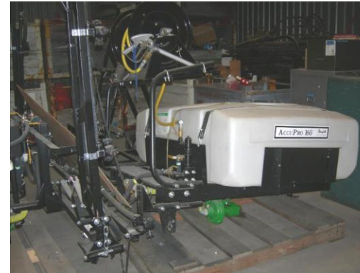
160 GALLON SPRAYER PORTION WITH BOOM FROM ACCUPRO UNIT
